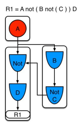
Figure 5.16. Example 4: Single rule, with sub-network and no sharing
